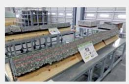
An actual sample of a pavement structure
