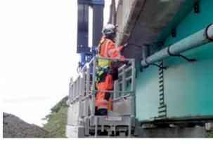
Conducting hammer tests on the bridge
