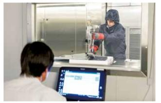
An accelerated corrosion testing apparatus
