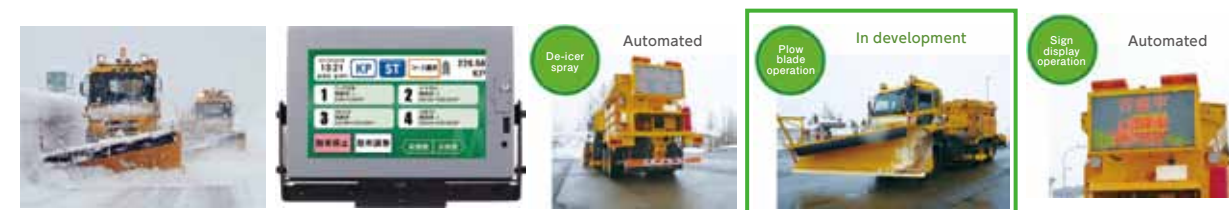
Automatic control by connecting to the high-precision positioning information
