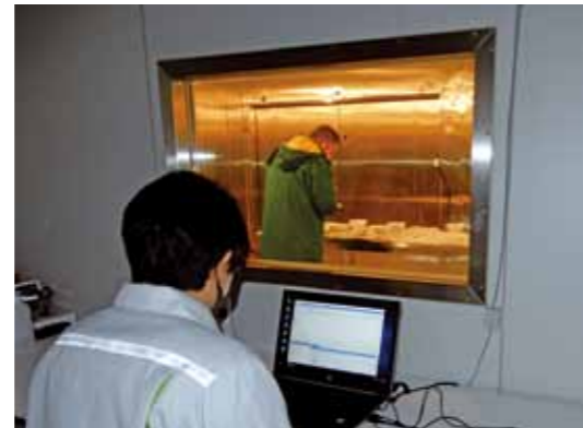
Antifreeze solidification test using the temperature and humidity test chamber
