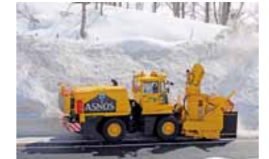
Autonomous driving test of a rotary snowblower on the main route
