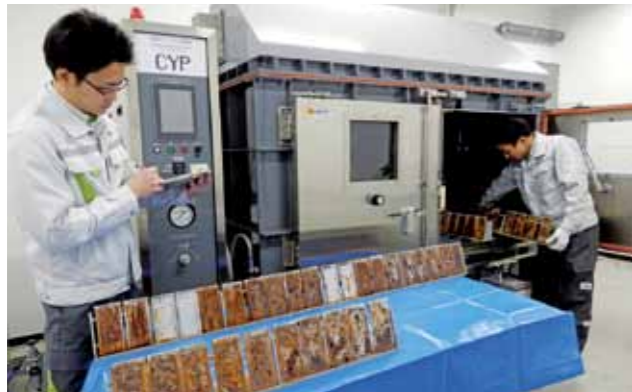
Material durability test using the accelerated corrosion testing device
