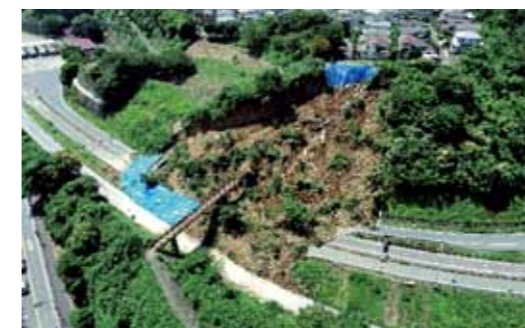
Zushi IC on the Yokohama-Yokosuka Expressway after the cut slope failure caused by heavy rain (left) and after resuming service (right)
