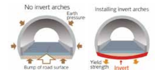
Image of countermeasure construction
