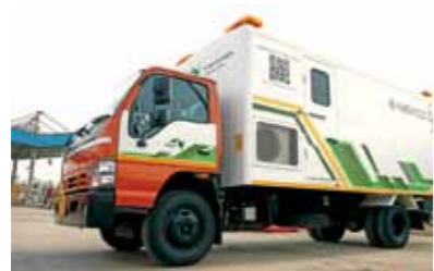
Road surface condition survey vehicle, E-NEXCO Eye
