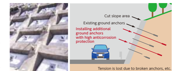
Image of countermeasure construction
