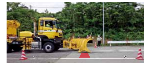
Automatic control by connecting to the high-precision positioning information
