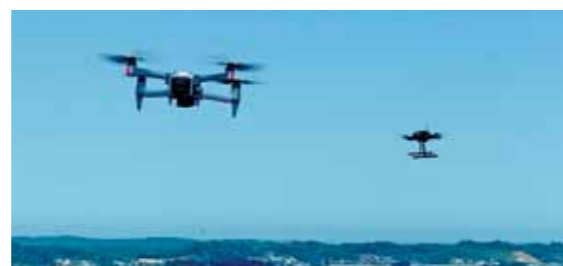
The back right drone automatically avoids another drone (front left).
