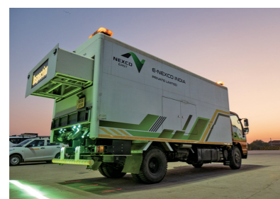
E-NEXCO Eye: Road surface condition survey vehicle
