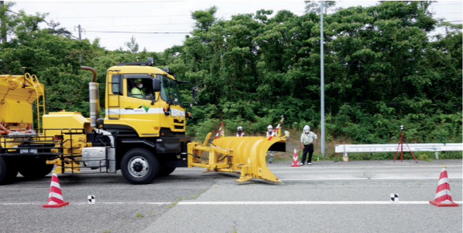
Automated operation of the plow blade in the test field at the Niigata Regional Head Office.
