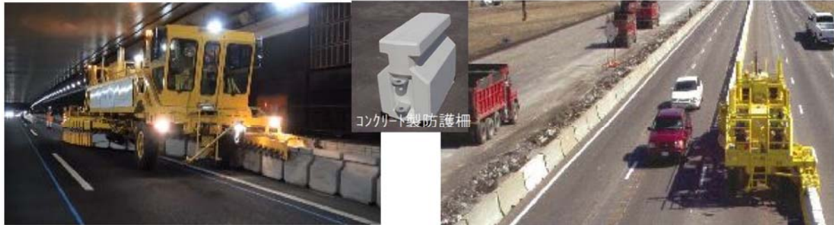
防護柵切替用車両:BTM (Barrier Transfer Machine)
