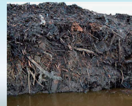
Cross section of tropical peat, bulldozed to make a highway in Brunei
